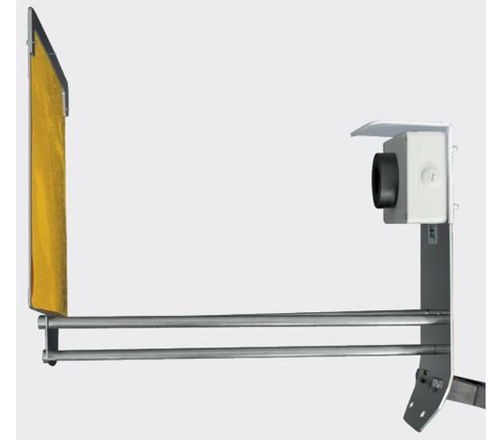
Thank you for choosing Pessl Instruments GmbH iMETOS iSCOUT® Color Trap for Remote Trap Image Monitoring. iMETOS iSCOUT® Color Trap periodically takes high resolution photos of the insect trap. Photos are automatically uploaded to the FieldClimate platform without the need of any user intervention, thus allowing a continuous insect control in the agricultural sector. Device comes with a high-resolution camera and a holder for a sticky plate.
