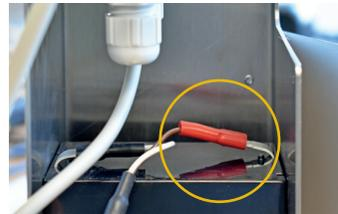
4. Connect the red cable to the positive battery terminal.
